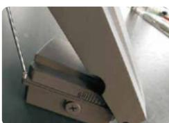
1. Remove screws and detach front of mounting box and fixture from rear portion of mounting box.
