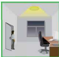
With insufficient natural light, the sensor switches on the light automatically when person enters the room. The lamp never switch off with presence, even the nature light is sufficient.
