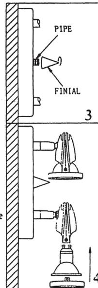
3. Tuck all electrical wires into the electrical box and install the light fixture to the wall by aligning the hole in fixture with the Pipe on the mounting bracket. Secure in place with finial.
