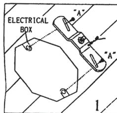
1. Assemble the mounting Bracket as drawing. Screw "A" into electrical box. The ground screw should then be attached to the mounting bracket (do not tighten).
