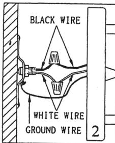
2. Attach the black wire from the light fixture to the black wire in the electrical box. Attach the white wire from the light fixture to the white wire in the electrical box. Connect the copper ground wire from the light fixture to the mounting bracket.
