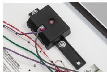
Simple adjustment of output through the use of a flat head screwdriver.
