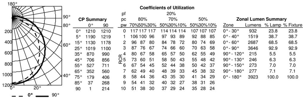
**BLWP4 40L ADP LP835**, 4391 delivered lumens, test no. ISF 37596, tested in accordance to IESNA LM-79.
