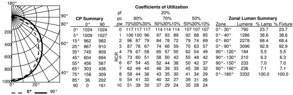
**BLWP2 40L ADP LP835**, 3923 delivered lumens, test no. ISF 37668, tested in accordance to IESNA LM-79.
