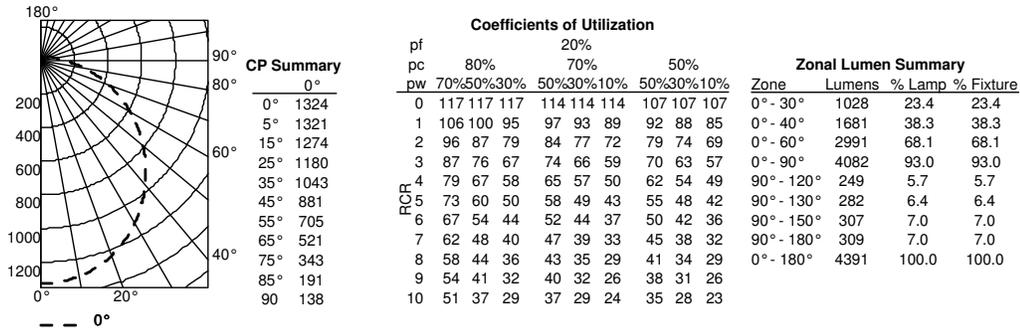
**BLWP4 48L ADP LP835**, 5137 delivered lumens, test no. ISF 37597, tested in accordance to IESNA LM-79.
