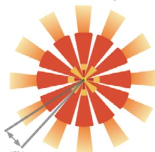
Lens rotates 15° to enable adjustment
