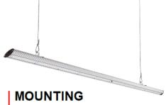
Suspend using conventional suspension cables or surface mount flush with junction box.
