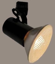
The AEH-00P00 can be used with Long Neck PAR30 lamps as well as PAR16, PAR20, and PAR38 lamps. Vertical slide adjustment slot allows numerous fixture heights. Half-yoke mounting design minimizes fixture presence. Precise, rigid aiming and full 350° horizontal rotation. Integral ON/OFF switch and track polarity indicator are standard.
