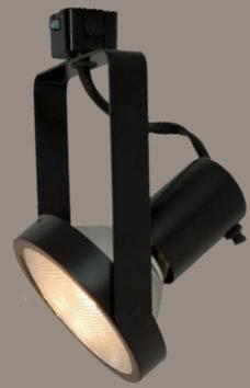
AEH-GBP38 has 2-plane gimbal design that allows 360° horizontal swivel and 150° adjustability in the vertical plane for excellent aiming. "Sure-Set" yoke holds the fixture firmly in place. Integral ON/OFF switch and track polarity indicator are standard.
