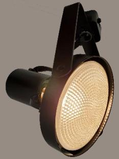
AEH-GFP38 has 2-plane gimbal design that allows 360° horizontal swivel and 150° adjustability in the vertical plane for excellent aiming. "Sure-Set" yoke holds the fixture firmly in place. Integral ON/OFF switch and track polarity indicator are standard.
