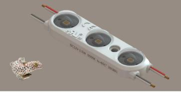
The GECO MFW1E3D1 from Aeralux is a compact and low profile LED SIGNAGE LIGHT designed for edge lit applications. This enables these modules to be suitable for channel letters with a 6-25 cm /2.4 - 9.8 in. depth. These also have great heat dissipation to ensure long life expectancy.
