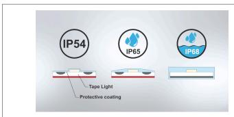
When using standard snap connectors, it is recommended to scrape off the coating from each conductor to ensure a proper connection. When using heavy duty snap connectors, this is only necessary for IP65 and IP68 types.
