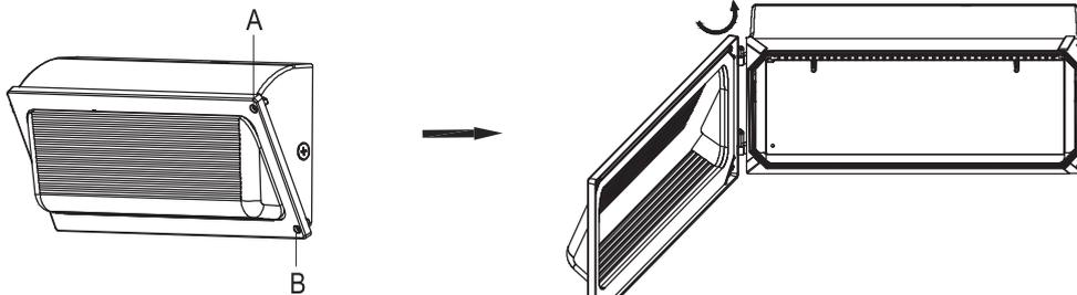
Loosen the 2x M5 screws (A/B) and open the fixture.
