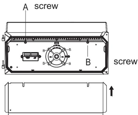
Put back the reflector and tighten the 2 screws
