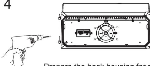
Prepare the back housing for mounting by drilling or knocking out the appropriate hole.
