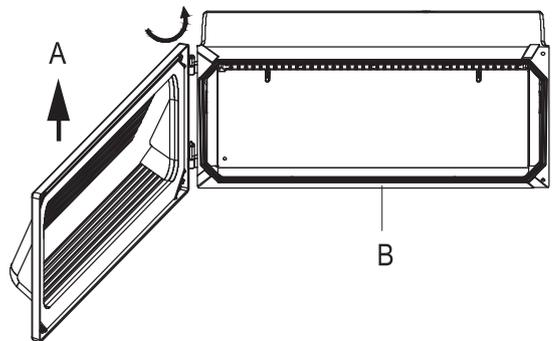
Put part A back onto the hinge of part B.
