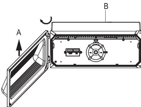
Separate part A and B and set part A aside.
