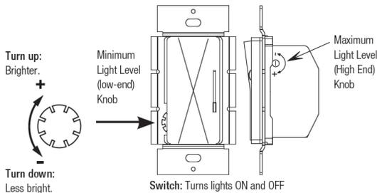
**IMPORTANT:** To avoid lights turn off or flicker at low end: Push slide down. Turn the low-end knob clockwise until the lights remain on without flickering.
