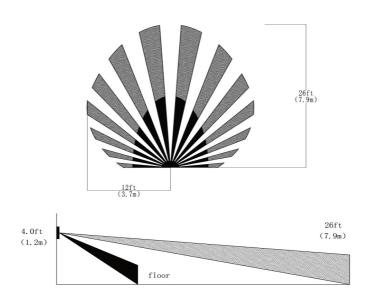
The detection area is measured under the best temperature condition of 20°C to 25°C. A higher temperature may not lead to an ideal detection area.
