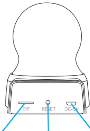
SD Card Reader    Reset Button    USB Power Supply
