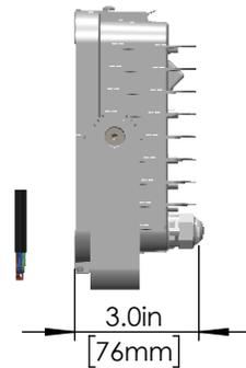
0-10V dimming wires must be run from a different conduit out of the J-Box.
