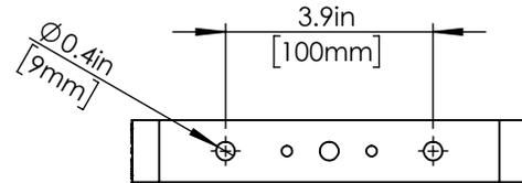
1. Locate, mark, and install anchors for the mounting bracket. Refer to the dimensions for the bracket as shown above.
