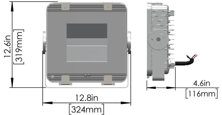
1. Install the fixture to designated location, and use dimension below for bolt's location.
