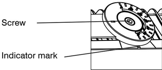
Loosen the screw to adjust the angle. Retighten once the angle is set.
