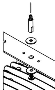
Press down to release lock. Release to engage lock.
