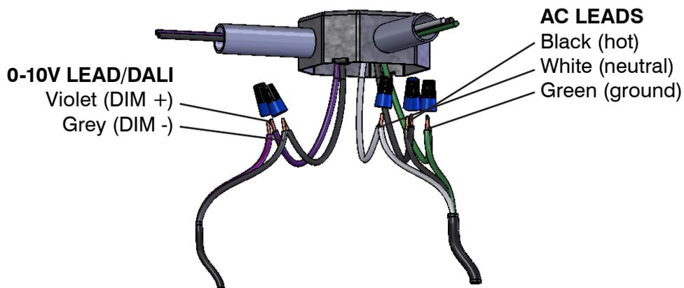
Note: For non-dimming, 3-conductor cord is available (upon request).
