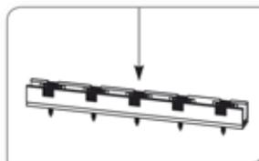
Put the grip plate into the groove of Aluminum track
