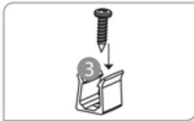
Screw the clip into the installation position
