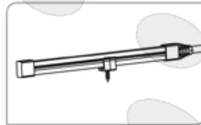
The tape light is flatly and firmly stuck in the clip
