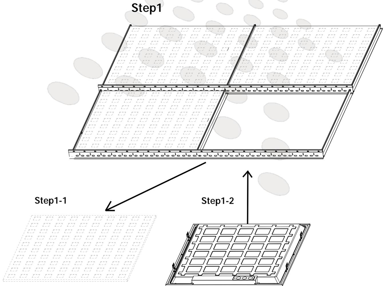
Step 1: Make sure of all the power is off before installing. Remove the one ceiling tile that you need to install light fixture on. Then place the light fixture on the T-bar carefully and make sure it is correctly in place and secure.
