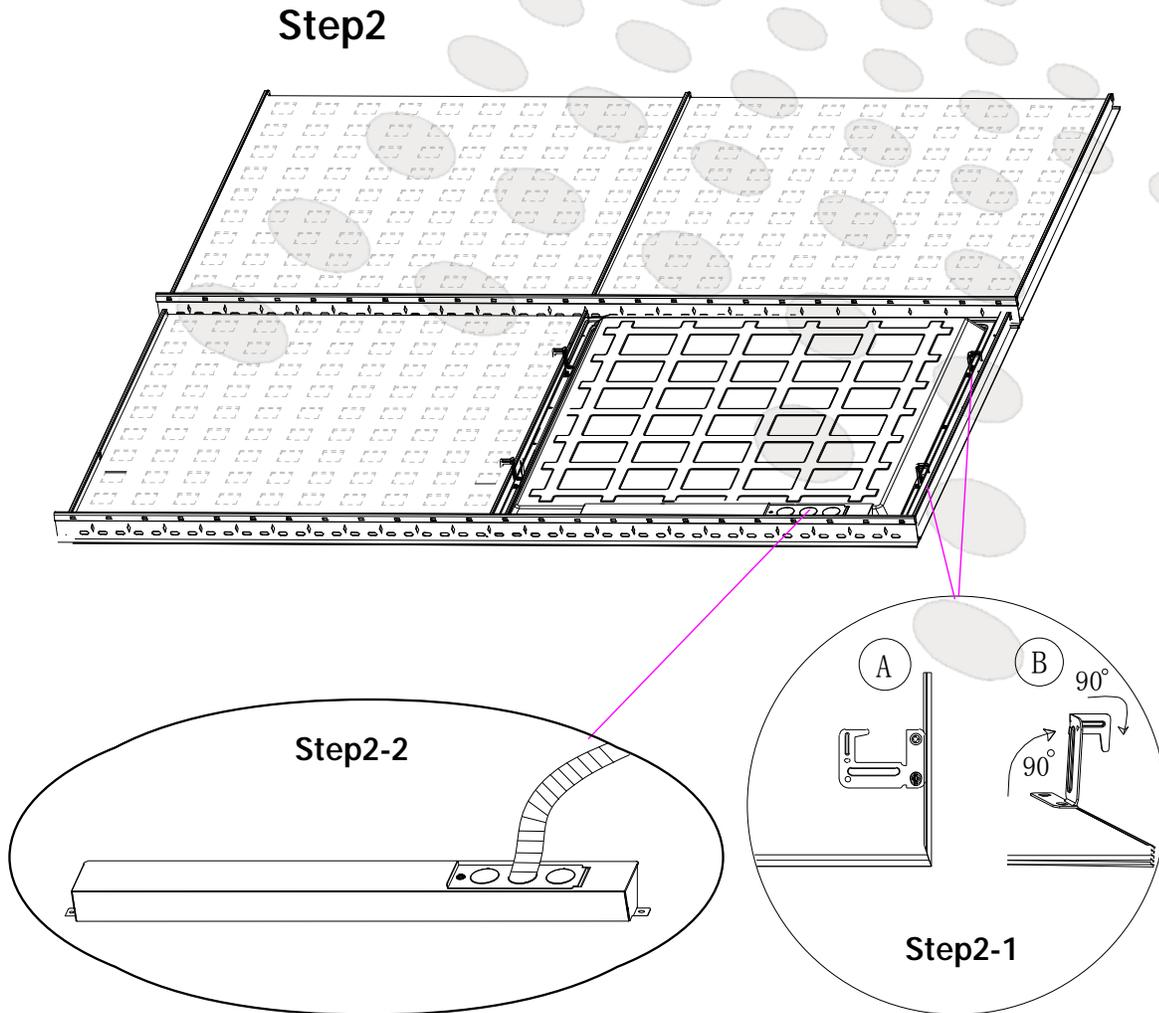
Step 2: Lift the 4 buckles on the back of the panel up by 90° then bend the top part of the buckles 90° towards the direction where you can anchor the light fixture to the T-bar.
