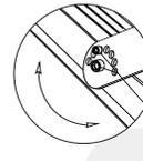
Loosen the angle to adjust the screw, after adjust to the angle that you need, then tighten the screws.
