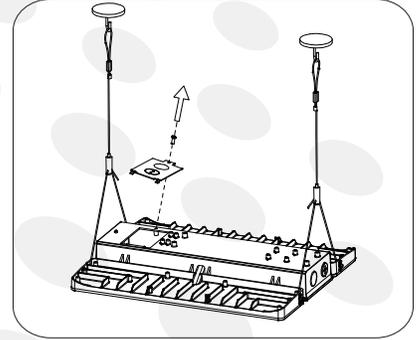
3. Remove the screws and remove the cover
