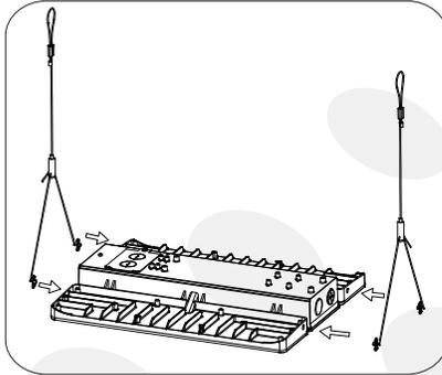
1. Install the lanyard into the light fixture
