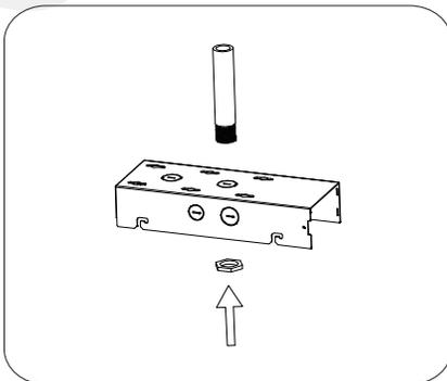
1. Install the junction box on the 3/4" pipe
