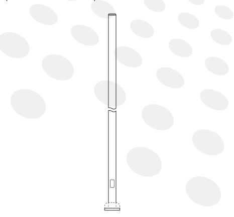
**Handhole:** 3 X 5 inches tall reinforced handhole is provided at 18 inches from the base. A cover with a single screw to secure the latch mechanism is also provided.
