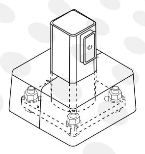
**Anchor Bolts:** A set of 4 galvanized steel anchor bolts is provided with each pole assembly. Each bolt includes 2 nuts and 2 washers. A portion of the anchor bolt is threaded for securing and leveling the pole with the provided nuts and washers. An actual size paper anchor bolt template is included.
