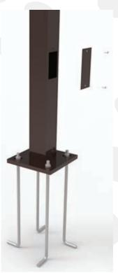
J-Type Anchor Bolts: A set of 4 steel J-Type anchor bolts are provided with each pole assembly. Each bolt includes 2 nuts and 2 washers. A portion of the anchor bolt is threaded for securing and levelling the pole with the provided nuts and washers. An actual size paper anchor bolt template is also provided.
