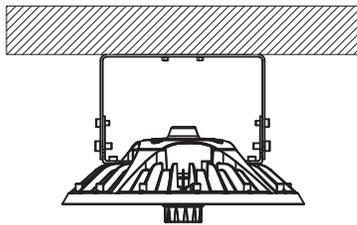
3. Fix the U bracket to the wall by nut, plain cushion, spring shim.
