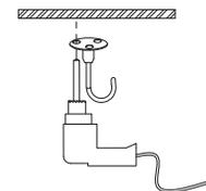
2. Use electric drill to bore a hole on the wall.
