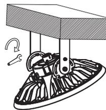
4. Use a wrench to reverse the hex nut and adjust the required angle.
