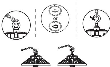
2. First fix the hook on the lamp (rotate clockwise) then connect the hook with the lock ring
