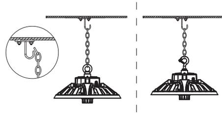
4. Fix one end of the chain to the wall, another end to the O/G hook from light, finish the installation.
