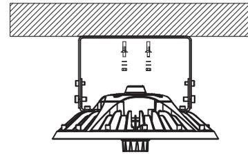
2. Install the expansion screw to the existing hole.
