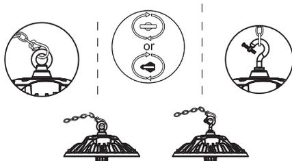
2. First fix the hook on the lamp (rotate clockwise) then connect the hook with the lock ring
