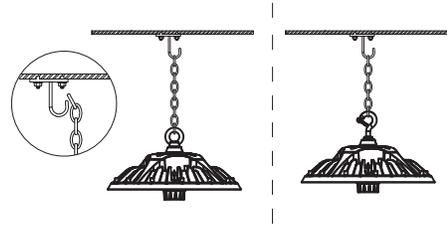
4. Fix one end of the chain to the wall, another end to the O/G hook from light, finish the installation.
