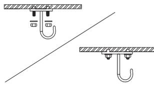
3. Fix the hanger on the wall with screws.
