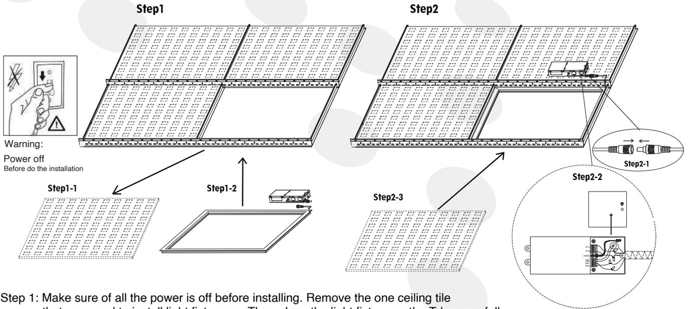
Step 1: Make sure of all the power is off before installing. Remove the one ceiling tile that you need to install light fixture on. Then place the light fixture on the T-bar carefully and make sure it is correctly in place and secure.
