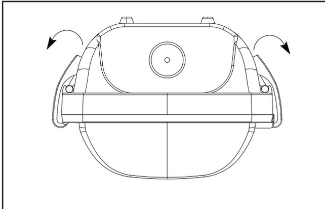
4. Without touching LED boards, detach LED tray and lens from fixture.
