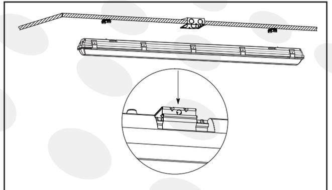
3. Release latches by pulling top of latch away from housing.
