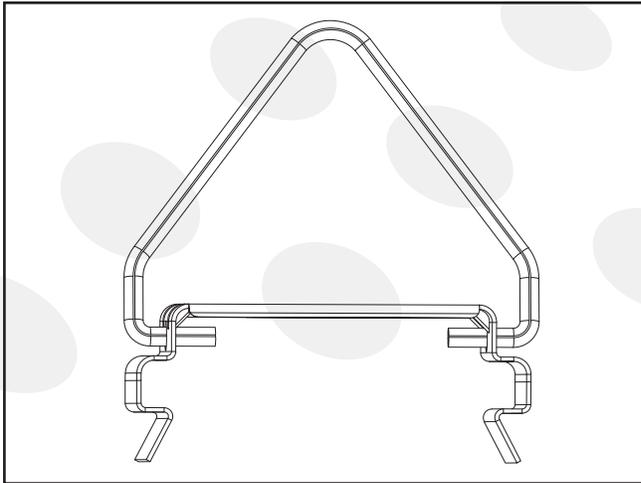
2. Secure mounting clips to housing recesses by firmly pressing them into place until both sides of the clip are secured. Hang fixture from customer supplied chain using V-brackets.
