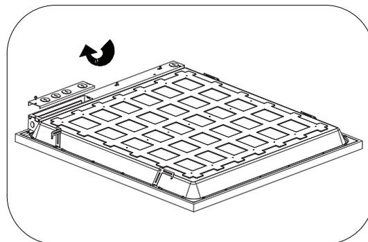
Remove electrical enclosure cover. Carefully remove knockout for AC line input wires and 0-10V control line. Install listed electrical fittings in the knockout holes for wire protection if needed.
