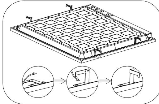
Lift up four mounting clips on the sides of the luminaire. You can do it by hand (Do wear work gloves) or use pliers
