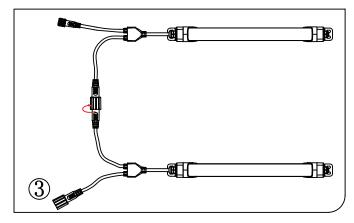
3. Tighten the nut of the connector.
