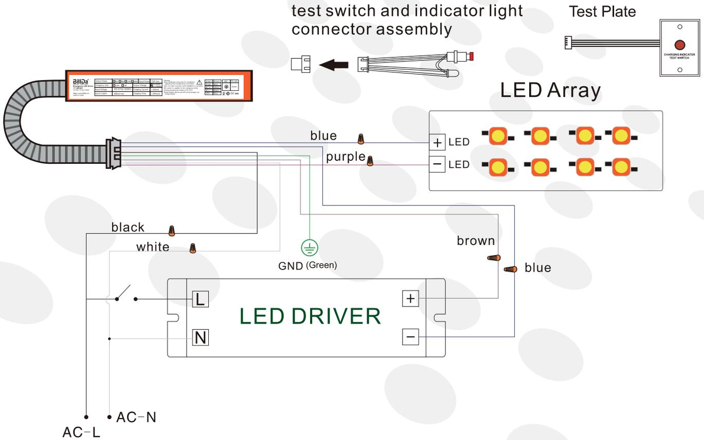
1. DO NOT MATE CONNECTOR UNTIL INSTALLATIONS COMPLETE AND AC POWER IS SUPPLIED
