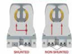
Shunted vs. non-shunted sockets Path of electrical current in red
