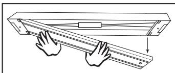
1. Remove the metal cover by loosening the screw.
