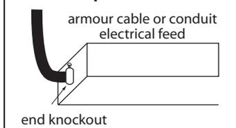
6. Alternatively, if an outlet (electrical) box is not available, if the fixture doesn't cover the outlet (electrical) box entirely or if the electrical leads are coming from either end of the fixture, please consult a qualified electrician for Armour Cable or Conduit Electrical Feed type of installation.
