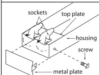
2. Locate the 2 pre-wired sockets from inside the housing. Remove the metal plate by loosening the screw. Push the sockets so that they snap into the slots on the top plate. Re-attach the metal plate to the housing by tightening the screw.
