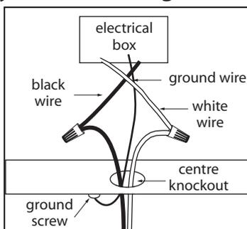
5. Connect the ground wire to the ground screw located near the center knockout. Connect the black wire from the fixture to the black wire from the electrical box. Connect the white wire from the fixture to the white wire from the electrical box. Once wires are connected, carefully tuck wires and marretts into the metal outlet box.
