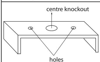
3. Turn the fixture over and locate the center knockout. Make sure the fixture is supported on the underside and break part of the knockout away using a hammer and screw driver. Twist out the knockout using pliers.
