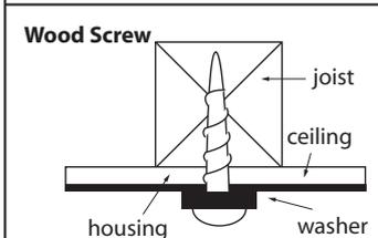
4. Position the housing on the ceiling with the center knockout over the electrical box. Mark the ceiling for the pilot hole locations through the small holes on either end. Drill 1/8" pilot holes at each location. Determine the appropriate way of fastening the fixture to the ceiling (wood screws or toggle bolts, not included). Note: Toggle bolts will require a larger pilot hole. Secure the fixture to the ceiling using the appropriate fasteners.
