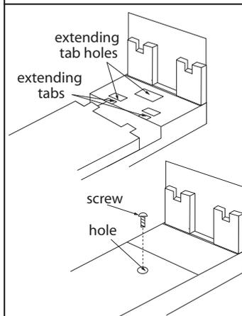
7. Re-attach the metal cover to the housing. Slide the end with the 2 tabs into the 2 holes at the end of the fixture and position the wire cover onto the fixture. Secure in place using the same screw removed earlier.
