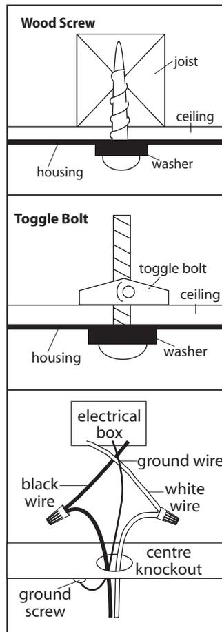
**5.** Connect the ground wire to the ground screw located near the center knockout. Connect the black wire from the fixture to the black wire from the electrical box. Connect the white wire from the fixture to the white wire from the electrical box. Once wires are connected, carefully tuck wires and marretts into the metal outlet box.
