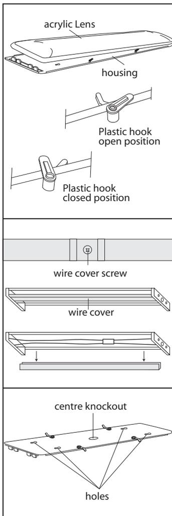
**1.** Remove the acrylic lens from the housing and place on a flat surface to avoid damage to the lens. To remove the lens release the four plastic hooks located 2 on either side of the housing from the closed position to the open position. Gently lift up the lens one side first followed by the other side.
