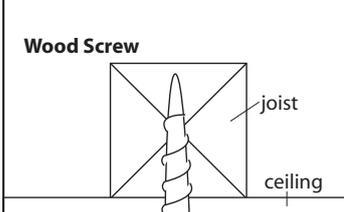
**3.** Position the housing on the ceiling with the center knockout over the electrical box. Mark the ceiling for the pilot hole locations through the small holes on either end. Drill 1/8" pilot holes at each location. Determine the appropriate way of fastening the fixture to the ceiling (wood screws or toggle bolts, not included).
