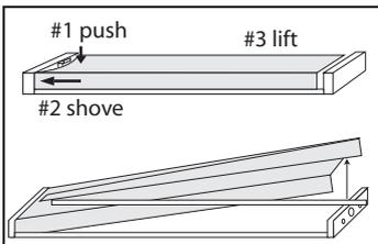
**1.** Remove the Acrylic Lens and place aside to avoid possible damage. Slide the lens towards one end of the fixture. Gently press down the end of the lens that is away from the housing. (Be careful not to crack the lens.) This will release the lens from the retaining clip. Lift up this end and pull the lens away from the fixture.
