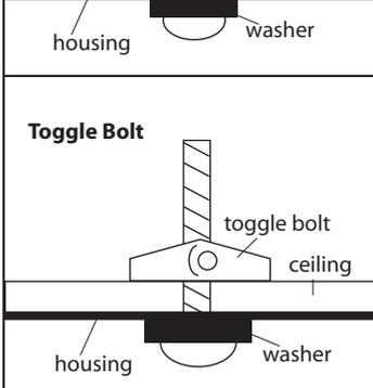
Note: Toggle bolts will require a larger pilot hole. Secure the fixture to the ceiling using the appropriate fasteners.
