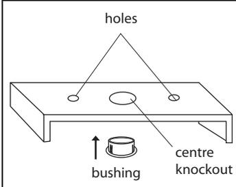
**2.** Turn the fixture over and locate the center knockout. Make sure the fixture is supported on the underside and break part of the knockout away using a hammer and screw driver. Twist out the knockout using pliers. Install the bushing as shown to the center knockout to protect the wires.
