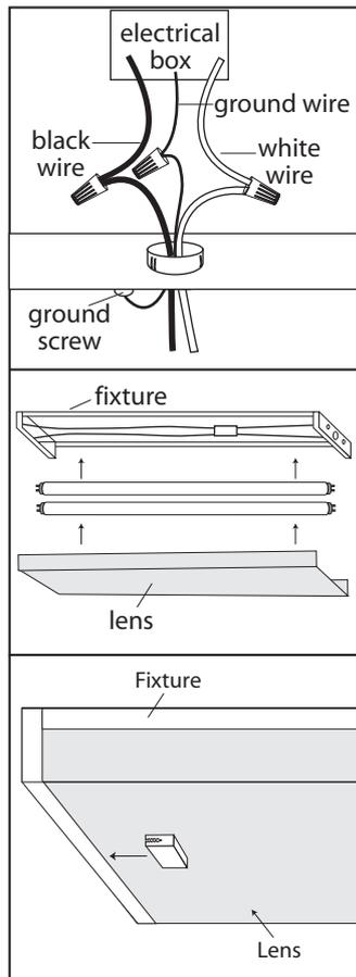
**4.** Connect the ground wires (bare copper or green) from your fixture to the ground wire (bare copper or green) or ground screw in the electrical outlet box. Connect black wire from fixture to black wire in outlet box and connect the white wire from fixture to white wire in outlet box. Once connections of wires are completed, carefully tuck wires and wire nuts into the outlet box making sure no bare wire (on the black and white) is visible at the wire nuts.
