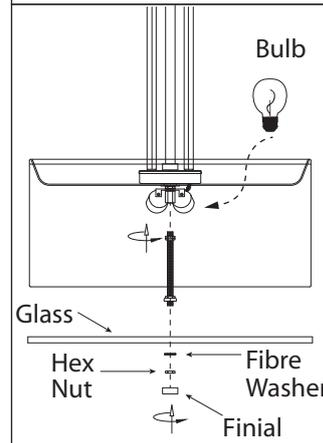
7. Attach the stem to the fixture. Secure the glass in place using the fibre washer, hex nut, and finial.
