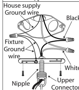
5. Connect the ground wires (bare copper or green) from your fixture to the ground wire (bare copper or green) or ground screw in the electrical outlet box. Connect the black wire (or wire marked "SPT-1") from the fixture to the black wire in the electrical box and connect the white wire from the fixture to the white wire in the electrical box.
