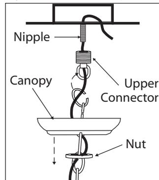
4. Loosen the nut on the upper connector and slide it down the chain towards the lower connector. Slide the canopy down the chain towards the lower connector. Feed the wire through nut, canopy, the upper connector and onto the nipple. Tighten the upper connector onto the nipple. Spread the other end of the chain open and fasten to the upper connector. Ensure the opening is closed.
