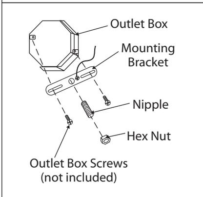
2. Attach the mounting bracket to the outlet box using electrical box screws (not included). Attach the nipple to the mounting bracket and adjust until it will clear the canopy when assembled (Place the canopy over the nipple and tighten the upper connector onto the nipple until snug. The upper connector should hold the canopy snug to the ceiling). Lock the nipple in the correct position using the hex nut.
