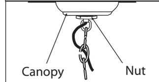
6. Once connections of wires are completed, carefully tuck wires and wire nuts into the outlet box making sure no bare wire (on the black and white) is visible at the wire nuts. Slide canopy into position and tighten in place by nut into position.
