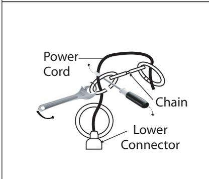
3. To attach chain loop to light fixture, use a screwdriver and wrench to open and close chain loop. Ensure to close the opening. Weave the power cord and ground wire through the links in the chain.
