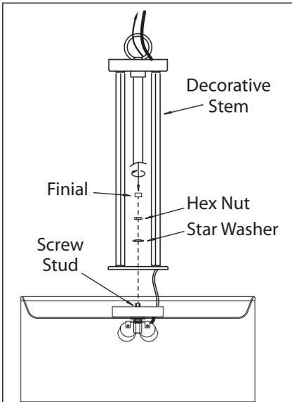
1. Slightly insert the decorative stem into the screw stud and tighten by a star washer, hex nut and the finial.
