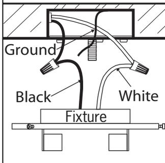
**2.** Connect the ground wire (bare copper or green) from your fixture to the ground wire (bare copper or green) or ground screw in the electrical outlet box. Connect black wire from fixture to black wire in outlet box and connect the white wire from fixture to white wire in outlet box.
