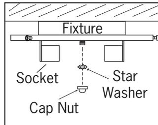
**3.** Tuck the electrical wires into the electrical box. Align the center hole in the fixture with the nipple in the mounting bracket. Secure the fixture in place with a cap nut.
