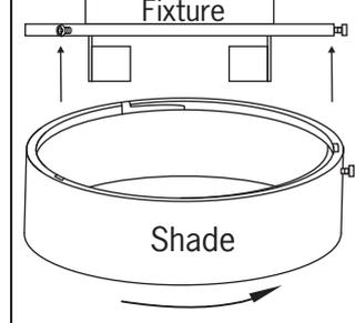
**5.** Push the shade upward and turn as shown. Lock the shade by tightening thumb screw against the fixture on the side.
