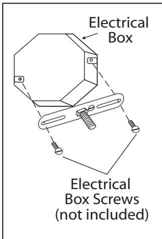
**1.** Attach mounting bracket to wiring box with wiring box screws (not included).
