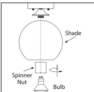
Remove spinner nut from socket. Position shade on lamp and secure with spinner nut. Install specified bulb type and wattage.
