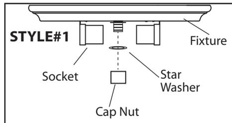
Align the center hole in the fixture with the nipple in the mounting bracket. Secure the fixture in place with a cap nut.
