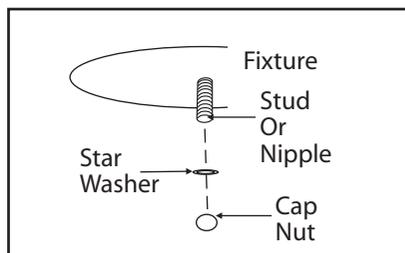
Tuck electrical wires into outlet box and position fixture over studs or nipple on mounting bracket assembly. Secure fixture in place with star washer(s) and cap nut(s).
