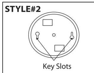
Tuck the electrical wires into the electrical box and position the "key slots" over the support screws. Turn and lock the support screws into the "key slots". Tighten the support screws into place.
