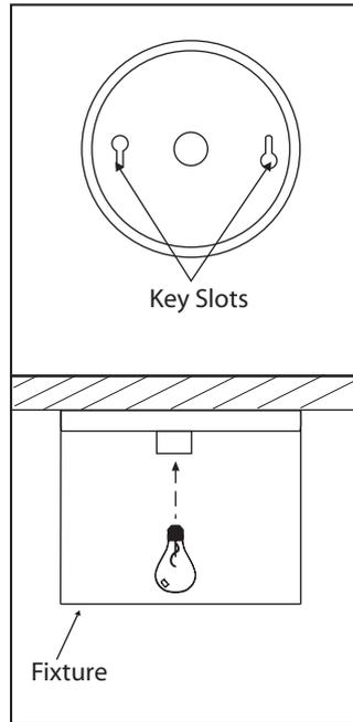
**3.** Once wire connections are completed, carefully tuck wires and wire nuts into the outlet box making sure no bare wire (on the black and white) is visible at the wire nuts. Tuck the electrical wires into the electrical box and position the "key slots" over the support screws. Turn and lock the support screws into the "key slots". Tighten the support screws into place.
