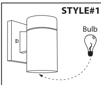
**STYLE#1** - Install specified bulb type and wattage (not included).
