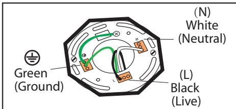
Connect (push) electrical wires from electric box (house wiring) into correct inserts. Black (Live), White (Neutral), Green (Ground)
