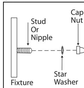
Tuck electrical wires into outlet box and position fixture over studs or nipple on mounting bracket assembly. Secure fixture in place with star washer(s) and cap nut(s).
