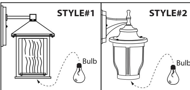
Install proper bulb type and wattage (not included).
