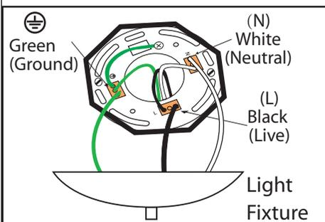
Connect (push) electrical wires from fixture into correct inserts. Black (live), White (neutral), Green (ground)
