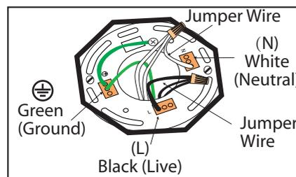
For multiple black (live) & white (neutral) wires joined in the electrical box (house wiring), attach a single "black" and "white" Jumper Wire before connecting. Strip 7mm from a 6" Jumper Wires (AWG 12-24) supplied. Then connect (push) wires into correct inserts.
