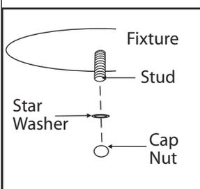
Tuck electrical wires into outlet box and position fixture over studs on mounting bracket assembly. Secure fixture in place with star washer(s) and cap nut(s). **Note:** If required, assemble body and spread the arms of the fixture out evenly.
