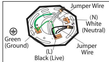
For multiple black (live) & white (neutral) wires joined in the electrical box, attach a single "black" and "white" Jumper Wire before connecting. Strip 7mm from a 6" Jumper Wires (AWG 12-24) supplied. Then connect (push) wires into correct inserts.
