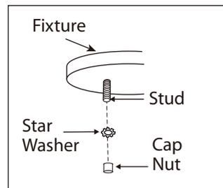
Tuck electrical wires into outlet box and position fixture over studs on mounting bracket assembly. Secure fixture in place with star washer(s) and cap nut(s).
