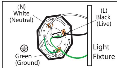
Connect (push) electrical wires from fixture into correct inserts. Black (live), White (neutral), Green (ground)
