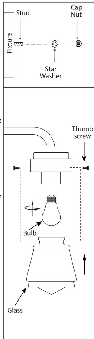
**4.** Tuck electrical wires into electrical box and position fixture over studs on mounting bracket assembly. Secure fixture in place with star washers and cap nuts.
