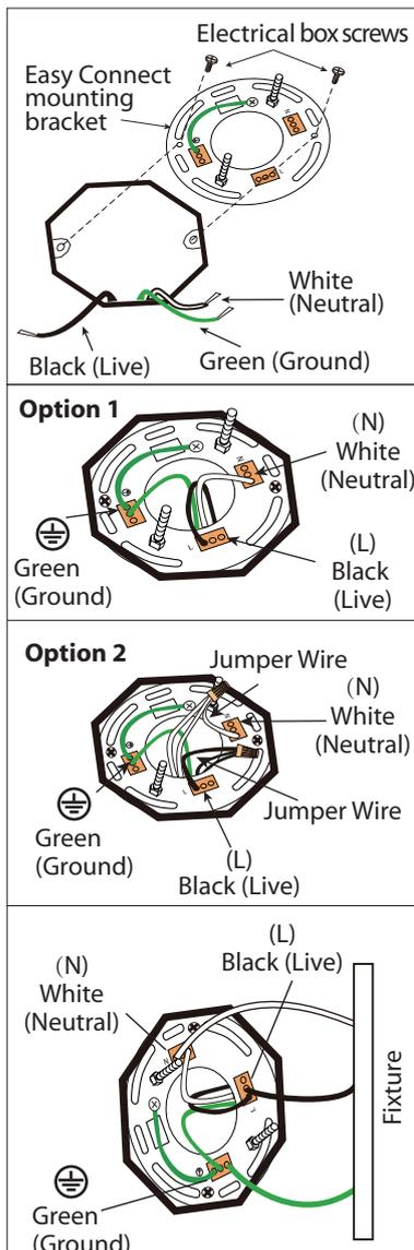
**1.** Attach easy connect mounting bracket to electrical box with electrical box screws (not included).
