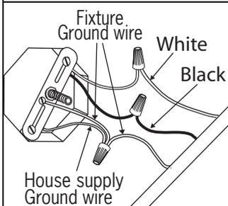
3. Connect the ground wire (bare copper or green) from your fixture to the ground wire (bare copper or green) or ground screw in the electrical outlet box. Connect electrical wires of fixture to wires in electrical box by marretting white wire to white wire, then black wire to black wire.
