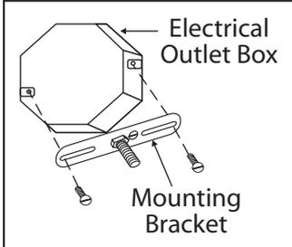
2. Attach mounting bracket to electrical outlet box with electrical box screws (not included).
