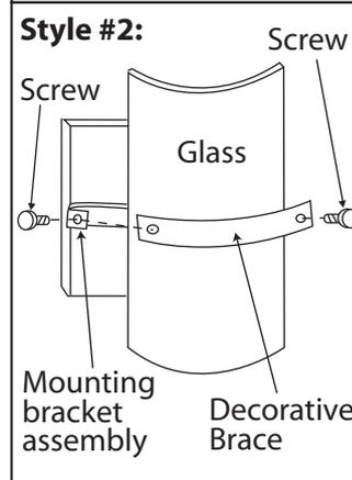
**Style #2:** Align glass and decorative brace to mounting bracket assembly. Secure in place with 2 (or 4) screws.
