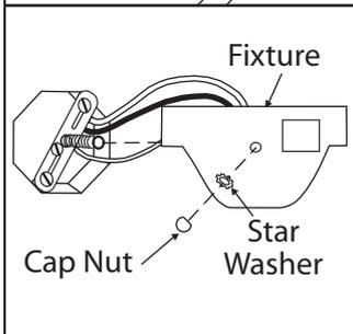
4. Tuck electrical wires into electrical box. Position hole in fixture over nipple and secure in place with cap nut.
