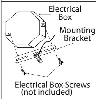
2. Attach mounting bracket to electrical outlet box with electrical box screws (not included).
