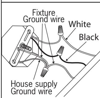
3. Connect the ground wire (bare copper or green) from your fixture to the ground wire (bare copper or green) or ground screw in the electrical outlet box. Connect electrical wires of fixture to wires in electrical box by marretting white wire to white wire, then black wire to black wire.
