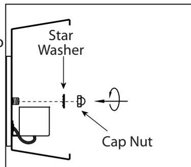
4. Once connections of wires are completed, carefully tuck wires and wire nuts into the electrical box making sure no bare wire (on the black and white) is visible at the wire nuts. Position hole in fixture over nipple and secure in place with star washer and cap nut.
