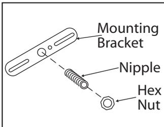
1. Attach nipple to mounting bracket. Adjust so it will clear hole in back of fixture and then lock nipple in place with hex nut.
