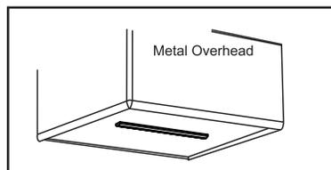
**2.** Attach the light fixture to desired position on metal shelf.
