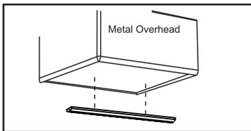
**1.** Attach magnetic mounting clips to the light fixture. Optimum clips location is 1" from each end of light fixture.
