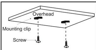
**1.** Plan your install. Pre-drill holes undercabinet. Install the mounting clips with the provided wood screws into predrilled holes. Make sure mounting clips are facing the same direction. Mounting clip optimum location is 1" from each end of light fixture (3/32" diameter x 1/4" deep predrilled holes)
