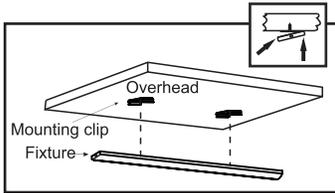
**2.** Raise the light fixture so the channel on the back aligns with the mounting clips.
