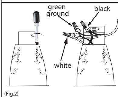
**2.** Unscrew the electrical box. Pull wiring through hole cut out. Using the wire-nut, connect the incoming and outgoing wires by matching white to white, black to black and green to ground wire and twist on. Tighten the electrical box after wiring connections. (Fig.2)
