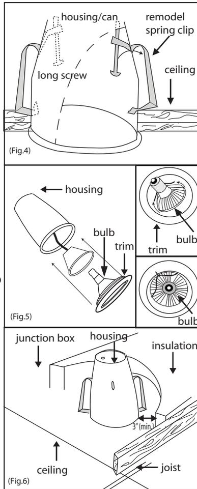
**4.** Screw the long screws against the back of the can. (Fig.4)
