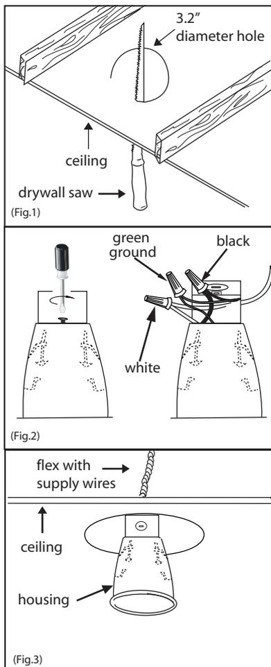
**1.** Using 3.2" template on the box, mark the openings and cut the openings with a drywall saw where you intend to install the lights. (Fig.1)
