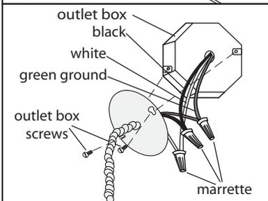
3. Connect the incoming and outgoing wires by matching white to white, black to black and green to ground wire and twist on. Install the joint box plate to the electrical outlet box with the outlet box screws. (Fig.3)
