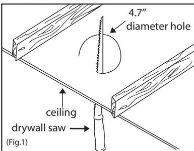
1. Using 4.7" template on the box, mark the openings and cut the openings with a drywall saw where you intend to install the lights. (Fig.1)
