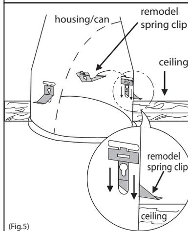
5. Push to lock the three remodel clips to hold the can against the ceiling. (Fig.5)
