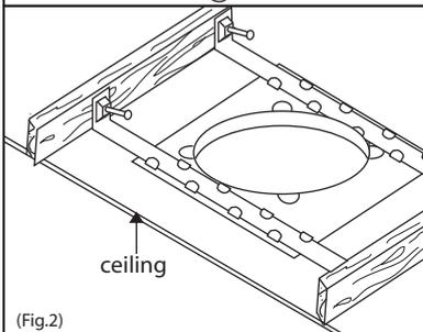
2. Spread the mounting bars (sold separately). Align the housing to the lower edge of the joists and hammer in place. (Fig.2)
