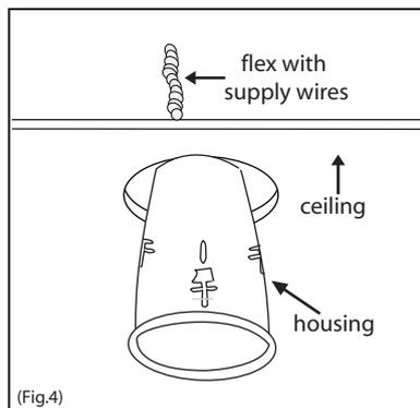
4. Lift the housing onto the drywall. (Fig.4)
