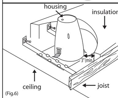
6. Do not install insulation within 76 mm (3 in) of any part of the luminaire. (Fig.6)
