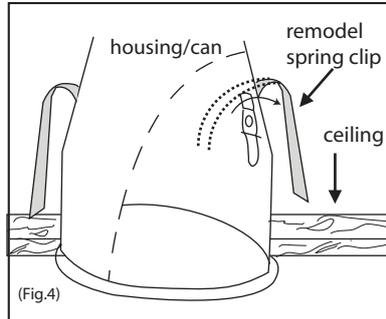
4. Push to lock the four remodel clips to hold the can against the ceiling. (Fig.4)
