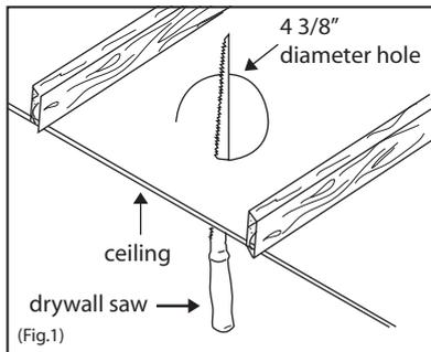
1. Using 4 3/8" template on the box, mark the openings and cut the openings with a drywall saw where you intend to install the lights. (Fig.1)
