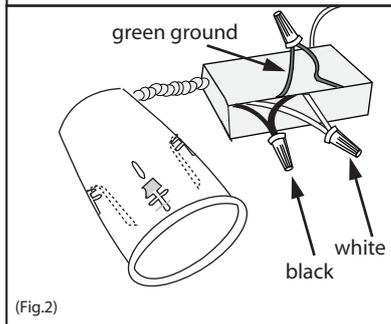
2. Pull wiring through hole cut out. Using the wire-nut, connect the incoming and outgoing wires by matching white to white, black to black and green to ground wire and twist on. (Fig.2)
