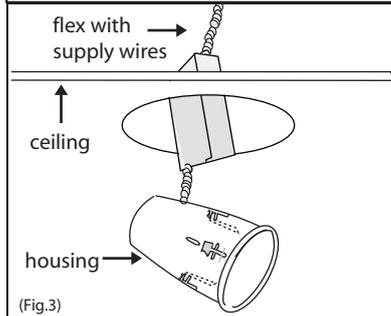
3. Lift the housing onto the drywall. (Fig.3)
