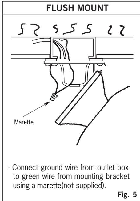
**NOTE:** Once ground wires are connected, carefully tuck wires and marette into the outlet box making sure that the wires are clear of the hemisphere and downrod when positioned in mounting bracket (Downrod Mount Only).
